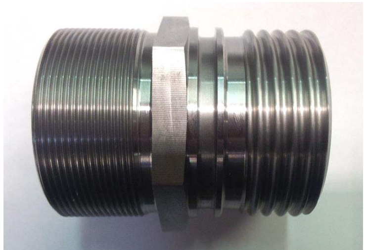
Connector, material C 45, dia. 3.74"-> 6flat WS 3.346", w=0.472"
